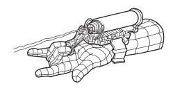
6. Place Web Blaster on forearm and fasten Velcro straps. Use middle fingers to press down on trigger to shoot web.
